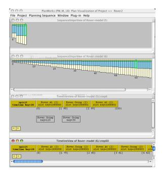
Figure 5: PlanWorks displaying data from two runs of the planner after modification of the model. The Sequence Step Views are shown at the top, and Timeline Views of the last plan step are shown at the bottom.
