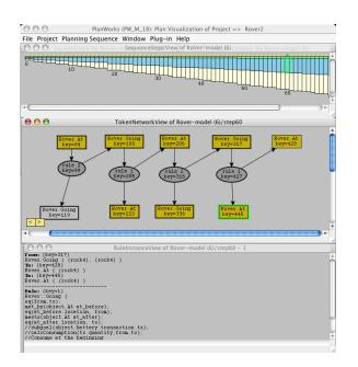
Figure 6: PlanWorks displaying a suspicious Sequence Step View (top), the long chain of rules (middle) and faulty rule in the Rule Instance View (bottom).
