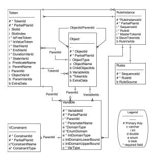
Figure 1: Part of the Entity Relationship Diagram for Plan-Works. This diagram shows the SQL table structure for Token, Variable, Constraint, Object, Rule and RuleInstance tables as well as the relationships between them.
